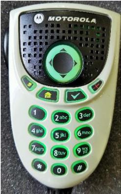
Mic number keys **1**, **2**, and **3** can be used to store a frequently used talkgroup or channel. It works like the memory buttons on a vehicle AM/FM radio.
