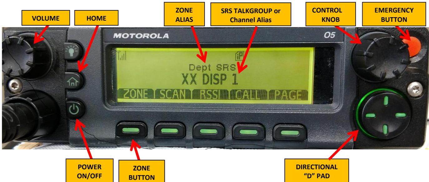
**Change Zone:** The radio can be programmed with a single “Zone” select button (shown above) or with separate “Zone Up/Zone Down” buttons. Zone Up/Zone Down buttons move directly to the next zone when selected. Pressing the Zone select button highlights the current zone. The Control Knob is used to cycle through the zone list. Pressing the Home button selects the desired zone.
